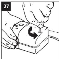
**Fixing Variable Signal Booster in permanent position.**
