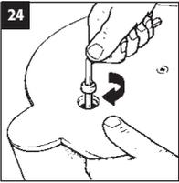
Secure Antenna Head **A** into position with Fixing Bolt and Nut **J** using Allen Key **K**.
