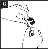
To re-fit connector, first strip away 15mm of the cable's outer sleeve. Gather the strands of copper screening and wind them back around the outer insulation.
