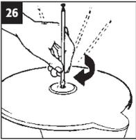
For vertically polarised and FM/UHF stations the Telescopic Antenna **G** should be added by first removing the screw, then screwing into Antenna Head **A**.
