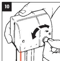
If a good picture cannot be received immediately turn the knob on Signal Booster **B** clockwise for more signal strength to optimise picture and sound quality. This knob can be rotated through six revolutions and will continue to rotate once you have reached maximum gain.
