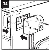
Assemble Booster unit with fixing screws after connecting coaxial and flyleads (see figs 6 and 8).
