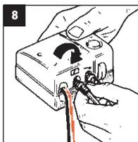
Connect one end of the 1 metre flylead **D** into the TV/FM socket on Signal Booster **B**.
