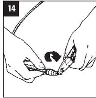
Feed the inner copper wire through connector and screw clockwise to tighten.
