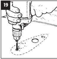
When drilling fixing holes we advise that you first use a much smaller drill bit, then drill the three holes with the appropriate size drill bit (2 x 8mm and 1 x 15mm).
