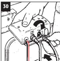
Connect to chosen power supply (see figs 2, 3 and 4 - OBSERVING SAFETY NOTES) and connect Coaxial Leads (see fig 6 and 8).
