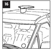
Mount the Gazelle antenna section as high as possible on a convenient surface outside the vehicle and place the associated booster inside so as to provide the best interference free TV or radio reception. In order to achieve the best possible interference free reception we recommend that the vehicle is parked well away from any overhead signal and power cables and away from any large physical obstructions such as trees etc.
