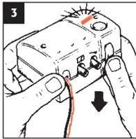
To supply power, push d.c. switch on the Signal Booster **B** downwards - the red light will illuminate.
