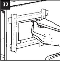
Alternatively, Signal Booster **B** can be panel mounted. Remove template from instructions and accurately cut out the centre rectangle. Use masking tape to fix the template to your chosen position, then carefully mark the cut-out area with a sharp pencil.
