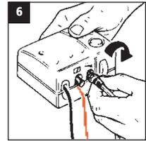
Screw the other end of 5 metre Coaxial Lead **C** into aerial socket on Signal Booster **B**.
