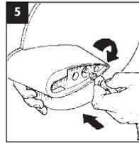
Connect screw connector on 5 metre Coaxial Lead **C** into base of Antenna Head **A** using integral box spanner to ensure a tight fit.
