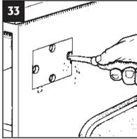
Drill a hole in the middle of each side of the template, big enough to take a jig or pad saw blade. Create the required rectangle by sawing from centre holes towards the corners. For dual voltage version, make a small rectangle to take the 230V mains lead (see template).
