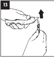
Strip away half the clear insulation around inner copper wire, checking that none of the screening wire is touching the inner copper core.
