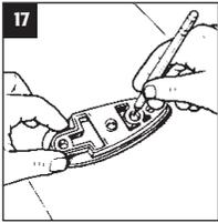
Use Mounting Base F as a template to mark the location of fixing holes for Antenna Head A.
