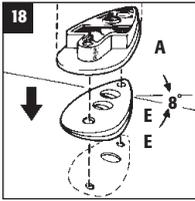
If the surface is angled use the angle pad(s) E provided to give the Antenna Head A a horizontal position.
