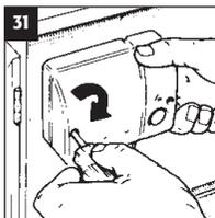
Replace casing on Signal Booster.
