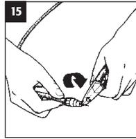
Cut off excess copper core to fit just above connector. **N.B** Recommended minimum length 1m.
