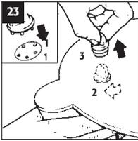
Use Security Key **H** to remove cap on Antenna Head **A** by turning 20 degrees clockwise and lifting.
