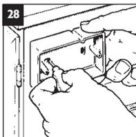
Use the back casing to locate a suitable position. Mark the two screw hole positions.
