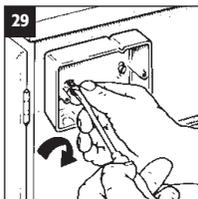
Fix back casing to your chosen location (fixing screws and wall plugs included inside casing).
