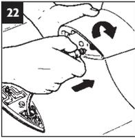
Push through screw connector on 5 metre Coaxial Lead **C** and connect into Antenna Head **A** (see fig 5).
