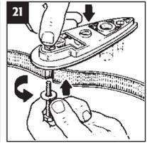
Fix Mounting Base onto your selected position using Roof Fixing Nuts, Bolts and Washers I.
