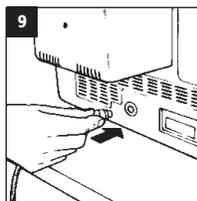
Connect the other end of 1 metre flylead **D** into the aerial socket on your TV and switch on in the usual way. Your TV should now be able to receive any transmitter, from any direction, within range.
